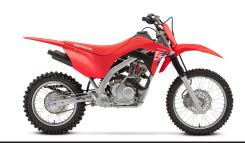
Engine Type 125cc air-cooled single-cylinder four-stroke
